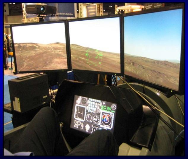
The Fighter application was built utilizing the EAAGLES framework. The heads down display was built by extending the provided graphics toolkit.
